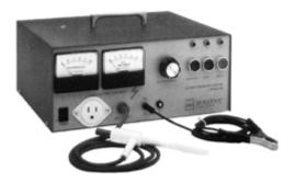
This Hi-Pot (Dielectric Strength) and Continuity tester is designed for production and quality-control testing. Perfor and Continuity testing on your products with a single tester. A practical tester for production testing in accordance and CSA. Available options provide compliance with IEC, TUV, and VDE as well.
